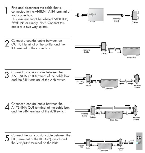
After you've made this connection, set the A/B switch to the "A" position for normal viewing. Set the A/B switch to the "B" position to view scrambled channels. (When you set the A/B switch to "B", you will need to tune your Set-Top Box to the cable box's output channel, which is usually channel 3 or 4.)
